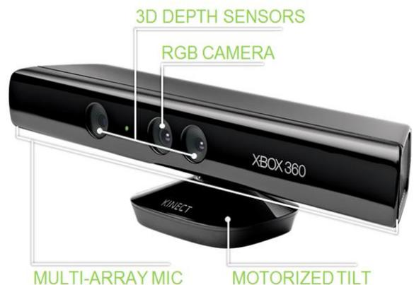
Fig. 1: Kinect Sensor
